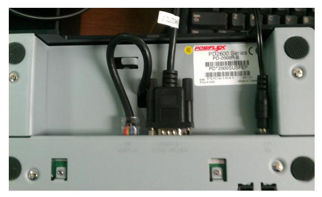
**Step 2:** Plug the serial port into the computer. Take note of which port you plugged into. If it is the only port, remember "COM1"
