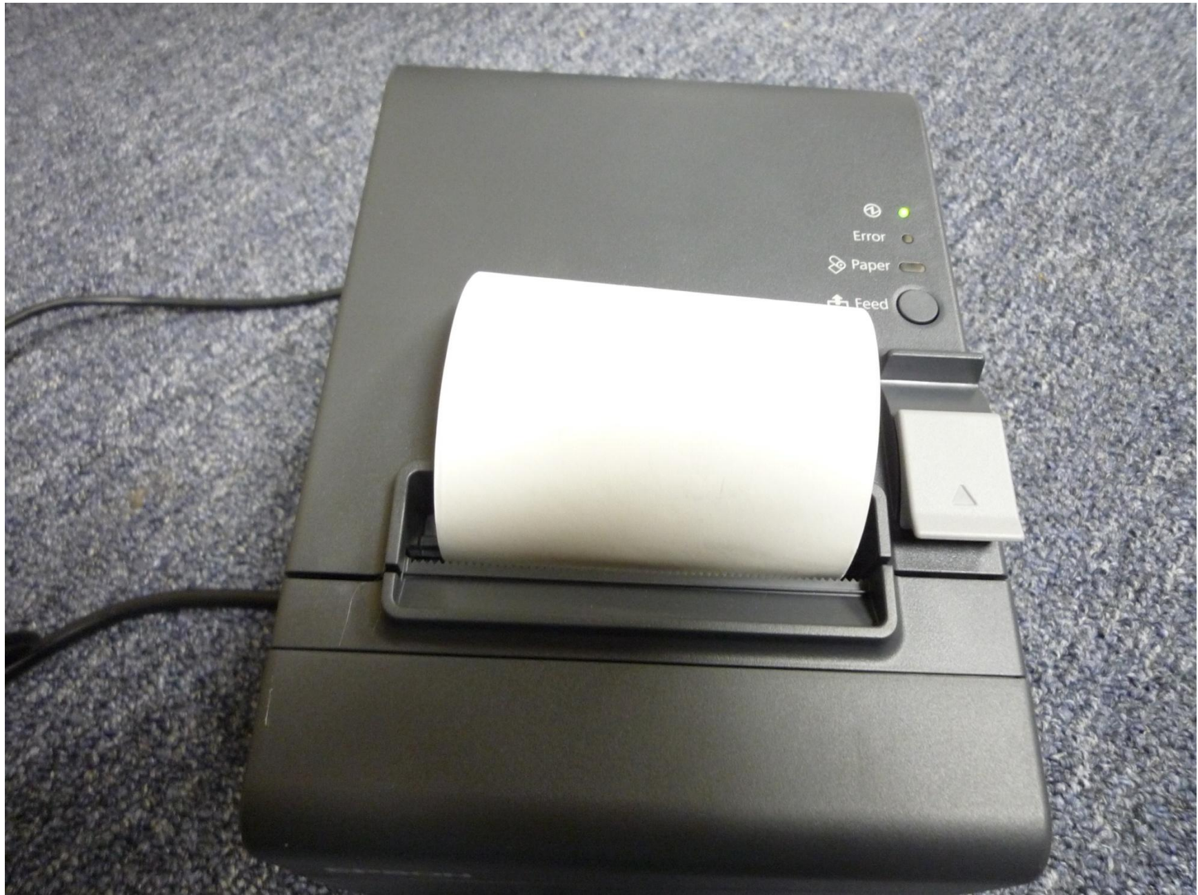
Properly connected receipt printer (Green light) with the cables and paper roll inside.
