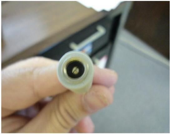
Cable 2b: This is connected with the serial port behind the CPU.
