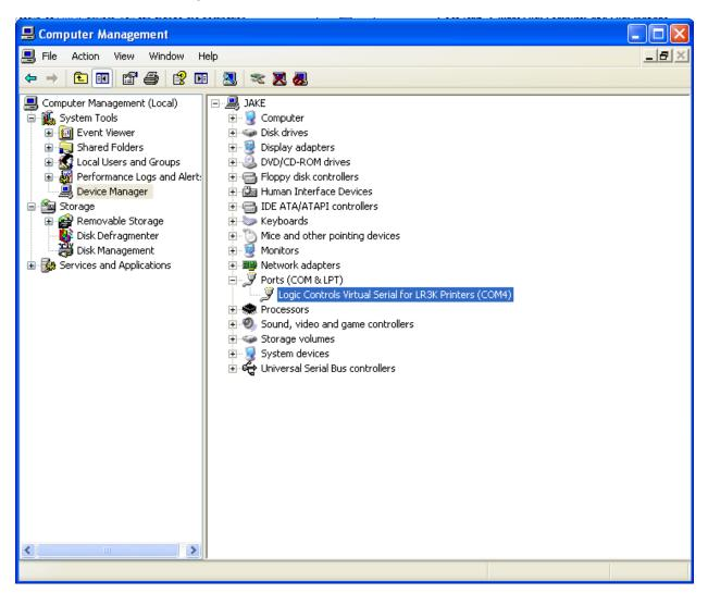
Open up the Logic Controls OPOS driver (Start -> All Programs -> Logic Controls PD OPOS -> Setup) Select the COM Port that was created.
