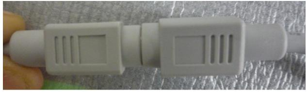
The figure shows the connection between **Cable 2a** and end of **power cable**.
